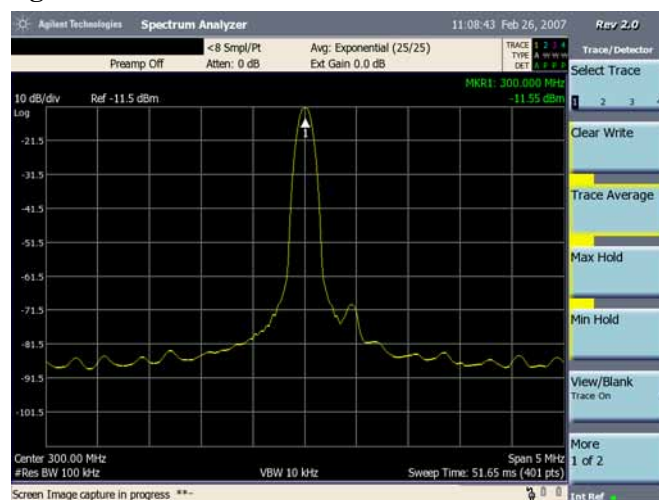
Figure 5-11 Signal Resolution with a 100 kHz RBW
