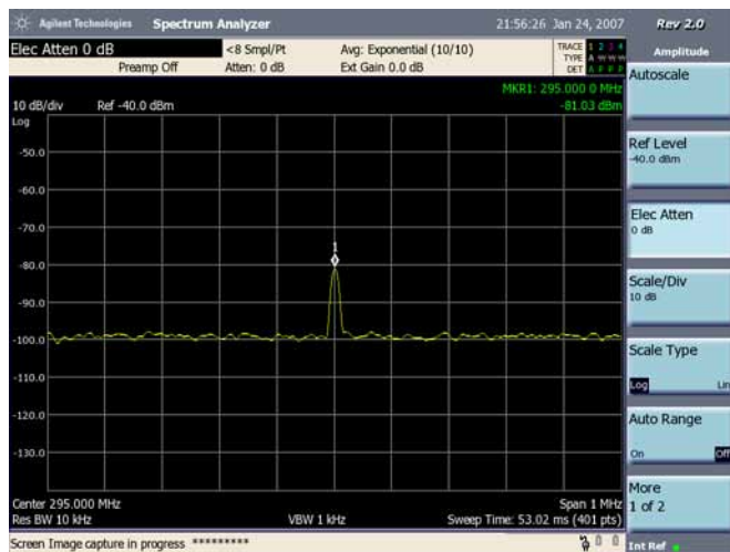
Figure 5-14 Measuring a Low-Level Signal Using 0 dB Attenuation
