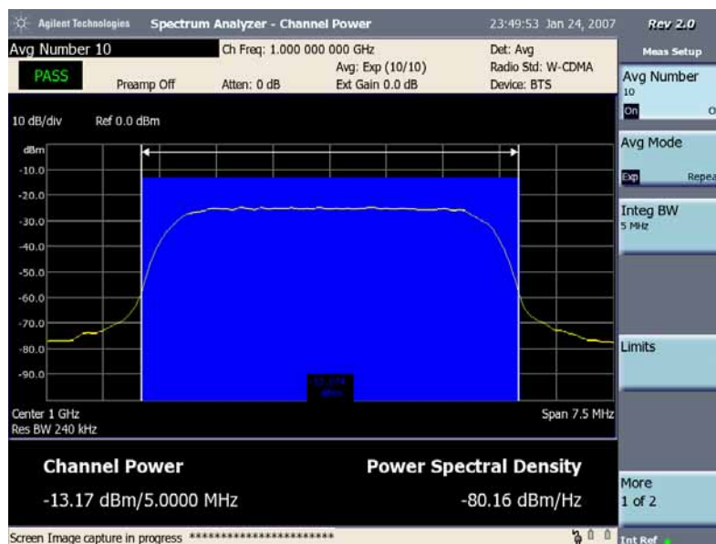
Channel Power measurement
