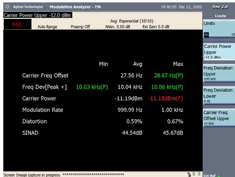
Figure 8-10 FM Numerical Results with Limits On
