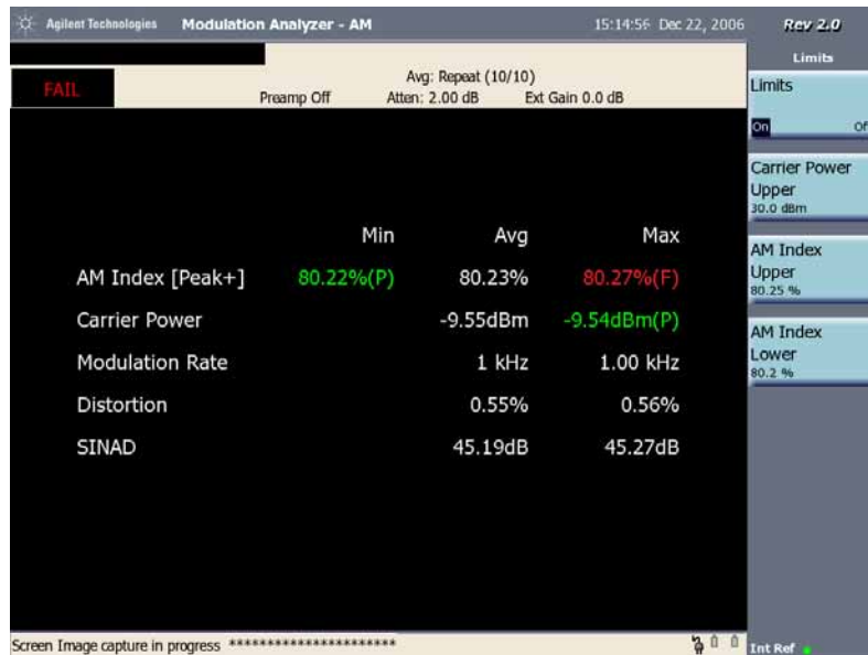
AM Numerical Results with Limits On
