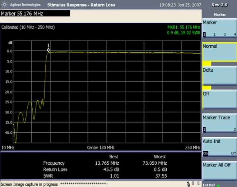
Return Loss Measurement Results, Calibrated.
