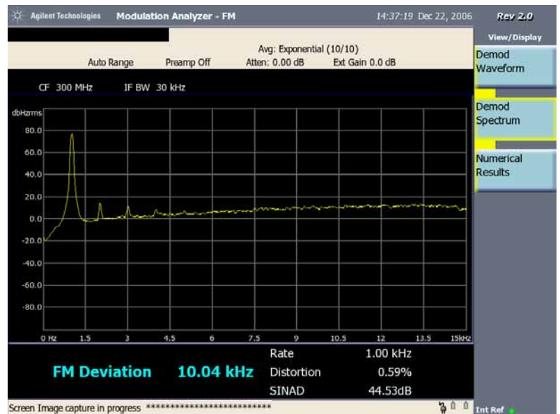
FM Demod Spectrum (ESG FM Signal with 10 kHz Deviation)
