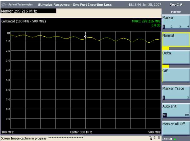
One Port Insertion Loss Measurement Results, Normalized.
