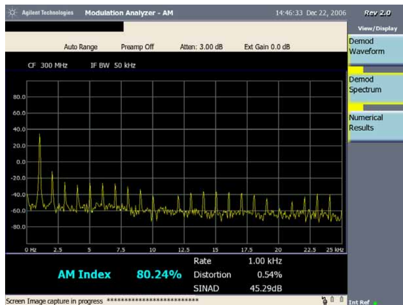
AM Demod Spectrum (ESG AM Signal with 80% Modulation Index)
