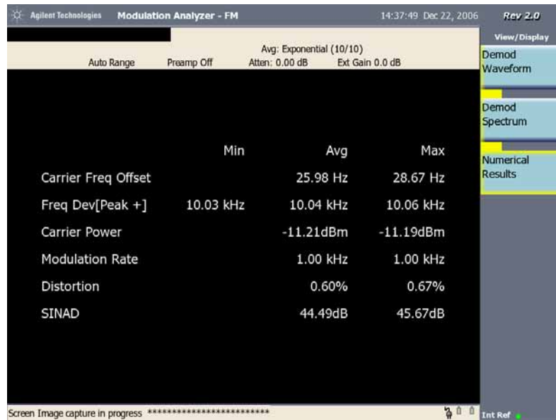
FM Numerical Results (ESG FM Signal with 10 kHz Deviation)
