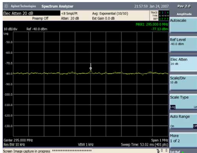
Figure 5-15 Measuring a Low-Level Signal
