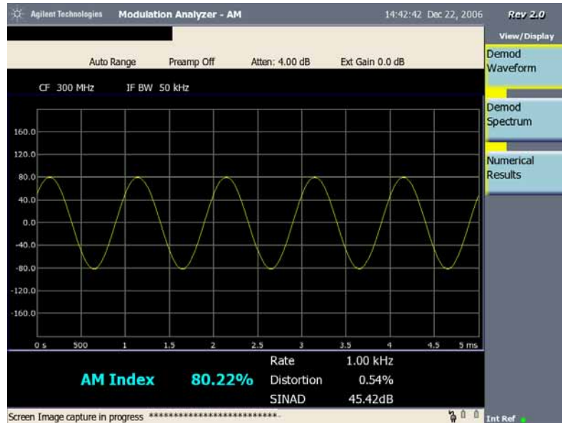
AM Demod Waveform (ESG AM Signal with 80% Modulation Index)
